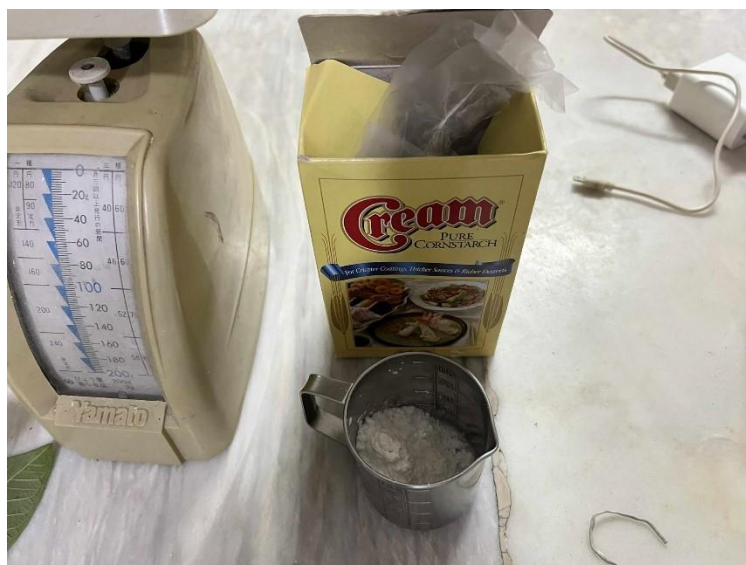
Figure 10. Cornstarch is measured as a natural binder to help hold the components of the corrosion inhibitor together.
