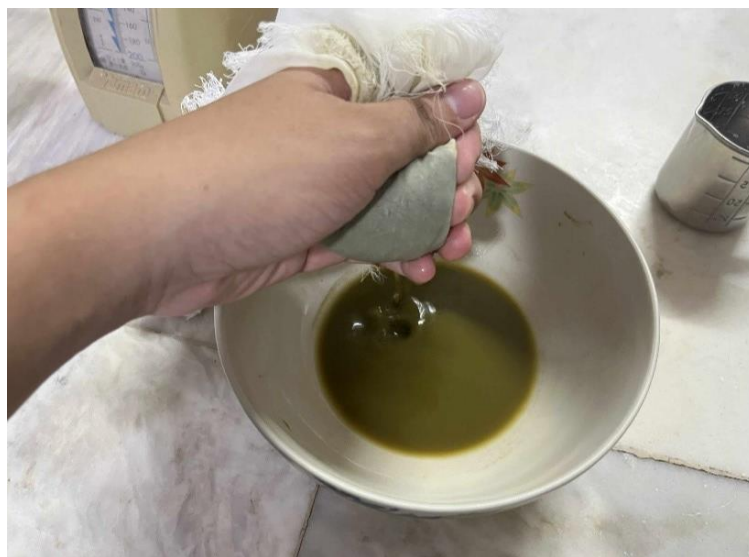
Figure 8. The boiled guava extract is strained using cheesecloth to separate the solid residues and obtain the liquid extract.
