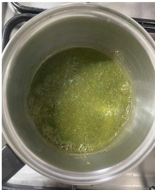
Figure 6. Ground guava leaves mixed with distilled water and subjected to boiling for 40 minutes to extract the plant's natural phytochemicals with corrosion-inhibiting properties.
