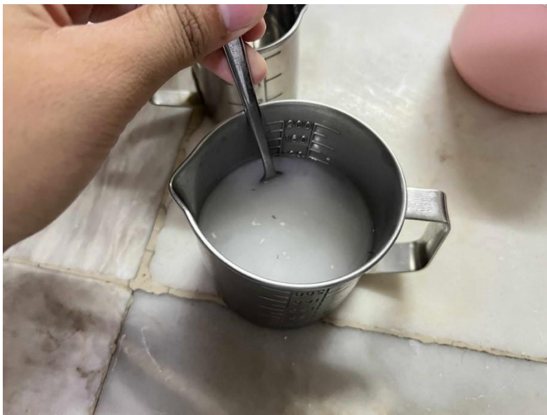
Figure 13. All components are mixed thoroughly and stirred continuously for 10 minutes to achieve a homogeneous corrosion inhibitor mixture.
