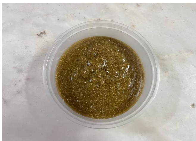
Figure 1. Guava leaf extract and Eggshell composite as a natural inhibitor for corrosion control.
