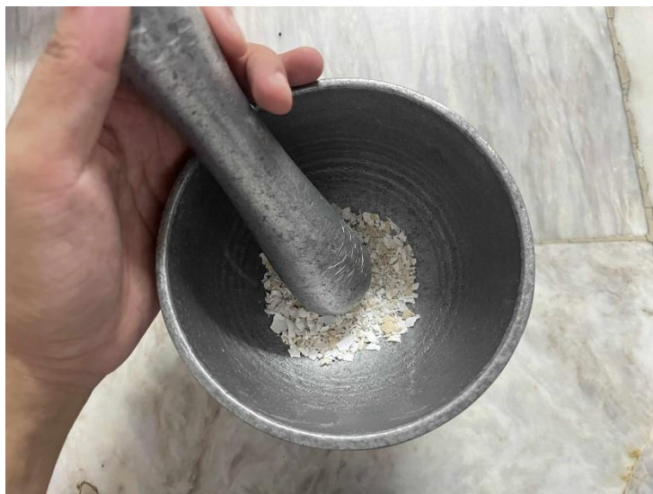
Figure 9. Dried eggshells crushed manually using a mortar and pestle to produce a fine powder for blending into the inhibitor formulation.
